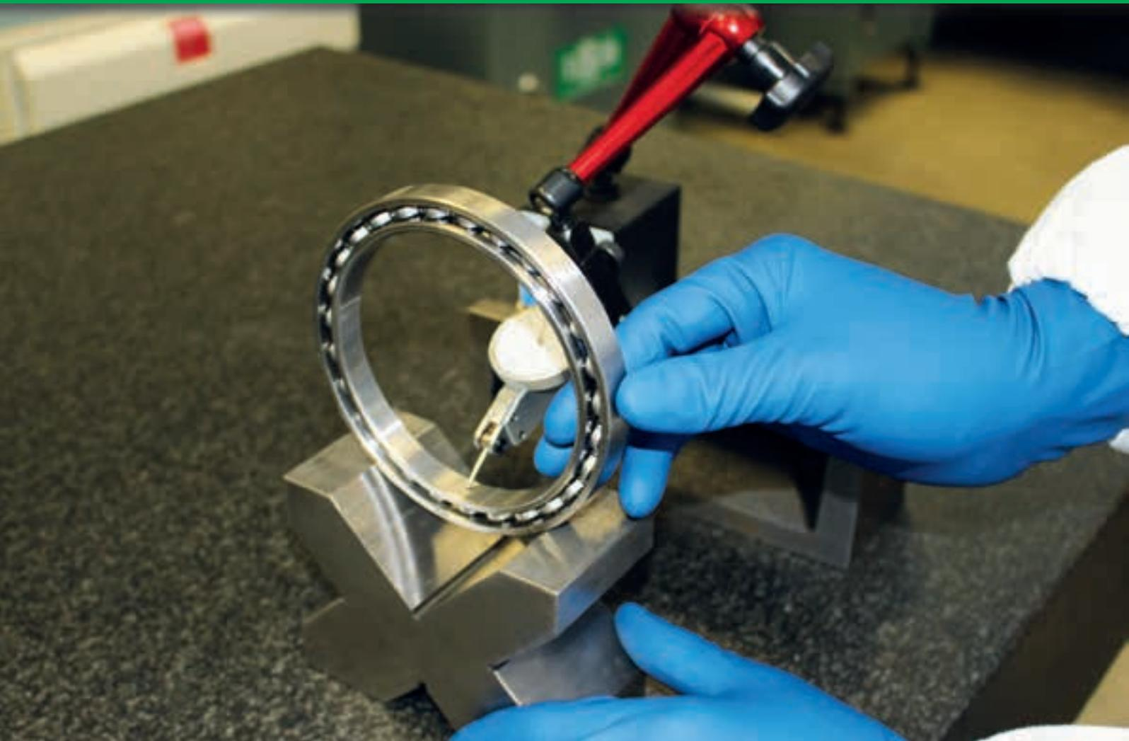
The correct installation of the bearing is an activity that does not start with the assembly phase of the component, but it is a complex procedure that consists of a series of phases whose improper, total or partial realization can cause problems with a consequent reduction of the calculated expected life of the bearing, that may be very relevant.
