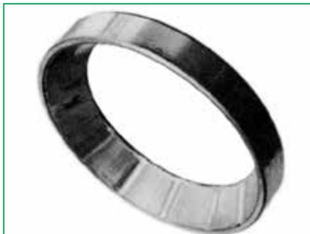
**Fig. 5****Plastic deformation, indentations on raceways spaced at rolling element pitch****Cause of failure:**
